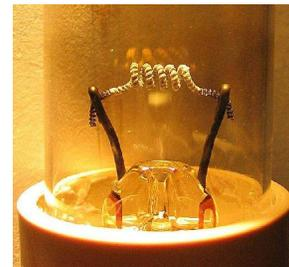
Fig. 2 Fluorescent light filament
