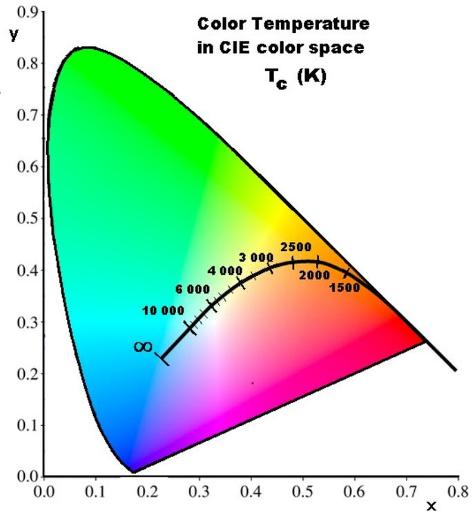
Fig. 11 Color Temperature for various BB temperatures
