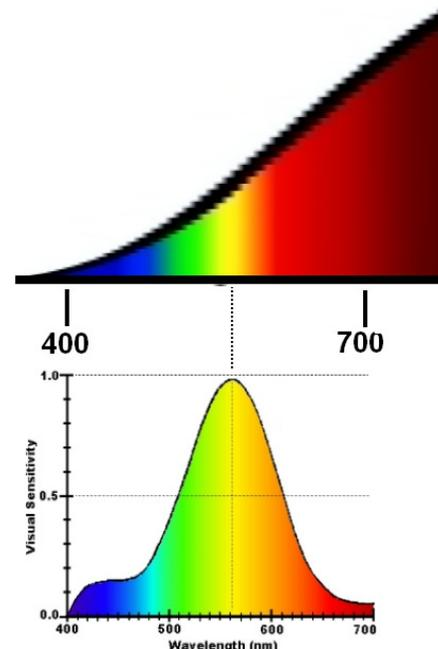
Fig. 10 Comparison of 2700 K bb emission and net sensitivity of eye
