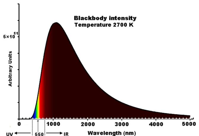
Fig. 9 Blackbody spectrum for an object at 2700 K temperature
